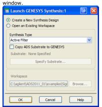
You need to specify whether you want to create a new design or open an existing Workspace. If creating a new Synthesis design, ADS asks what type of synthesis you'd like to perform and then launches GENESYS preconfigured to perform the synthesis.
